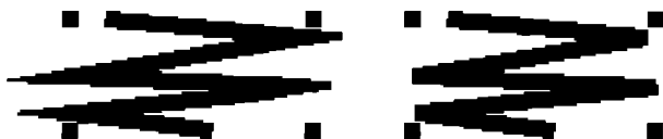
Figure 7. GraphicsContext join styles: joinMiter and joinBevel .
