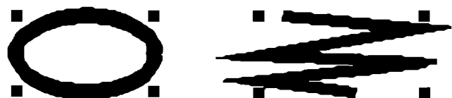
Figure 6. Thick lines and default join style extend beyond boundingBox.
